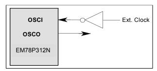
Fig. 5-29 Crystal/Resonator Circuit
